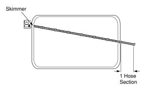
For center installations, connect enough hose to reach the farthest point of the pool and then add two more sections.
